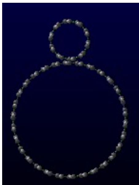
Figure 4: A side view of the two nanotubes that make up the transmission.
