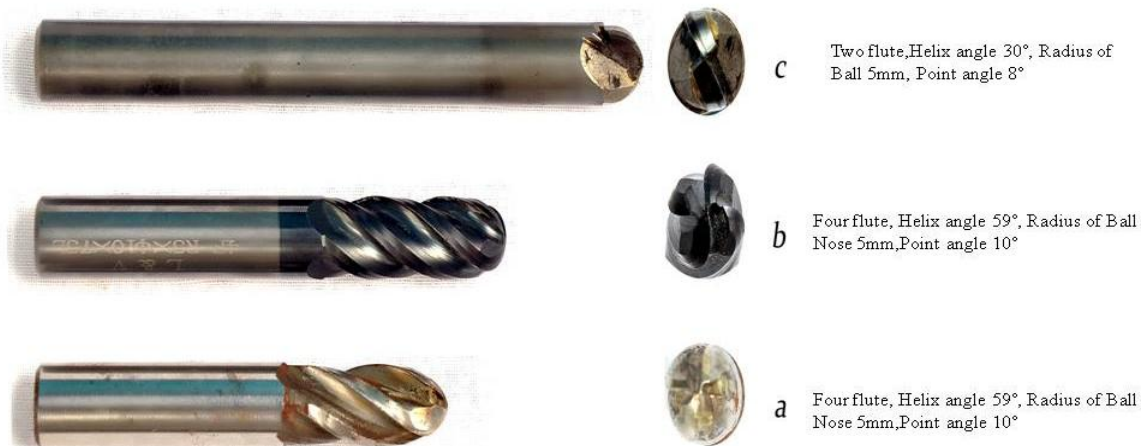
Fig. 1. Drills used in the study a) HSS Ball Nose, b) Carbide Ball Nose, c) PCD Ball Nose
