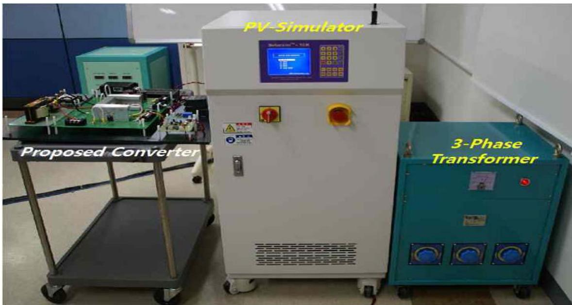
Fig. 12. Experimental setup using the Solarsim-10k PV simulator.
