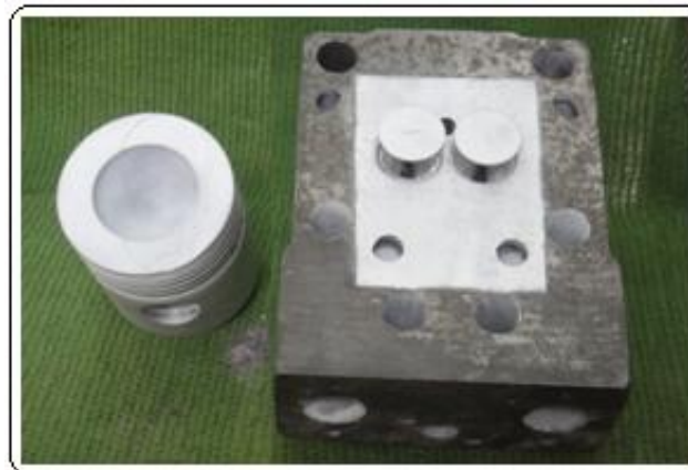
Fig.1 Photograph of PSZ coated piston, Cylinder Head and Valves
