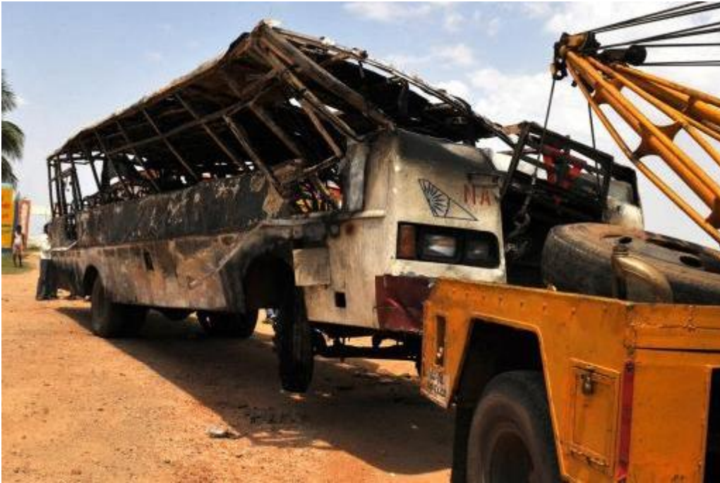
Fig.2 Damaged bus structure after rollover accident
