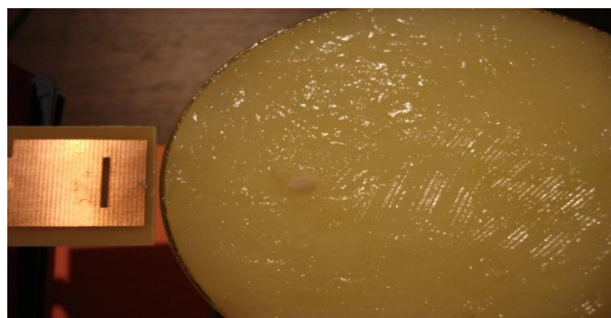
Fig. 9: Transmitter antenna and tumor placed inside breast phantom
