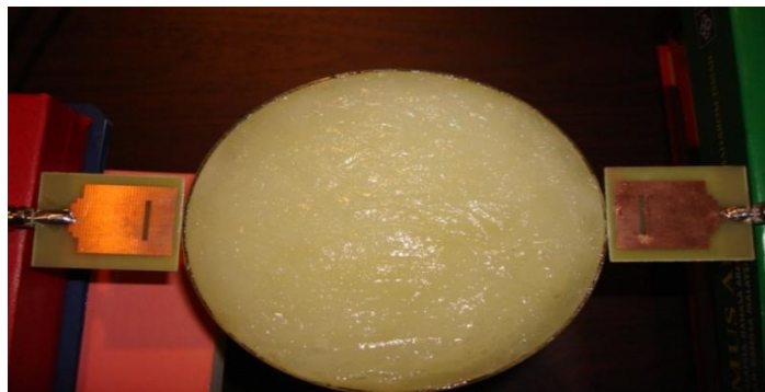
Fig. 8: The directional antennas during experiment setup
