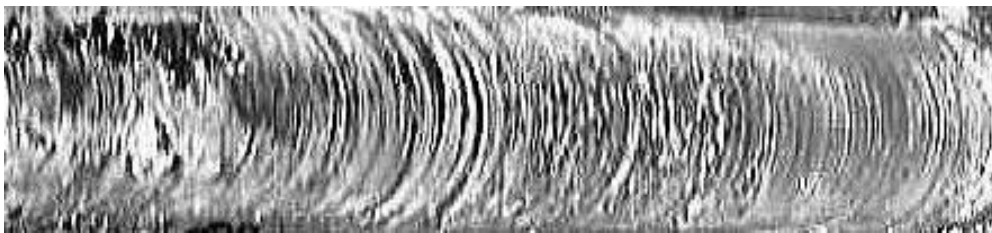
Fig.4: Gray Scale, Processed Weld Bead Image FSW Specimen 1
