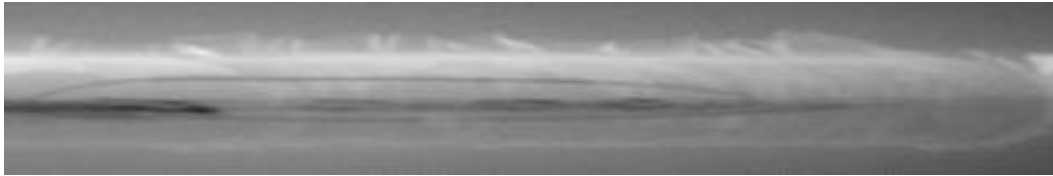
Fig.13: X-Ray Radiography of FSW Specimen 2
