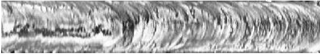
Fig.12: Gray Scale, Processed Weld Bead Image FSW Specimen2
