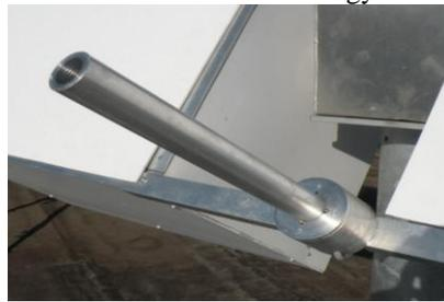
**Fig. 5:** Solar collimator for biaxial tracking
