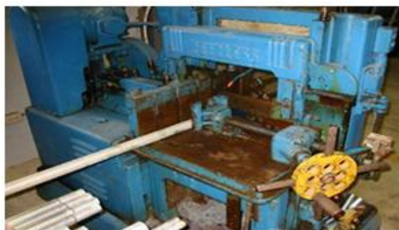
Figure 2- 5 Metal-cutter for cutting the work piece material.
