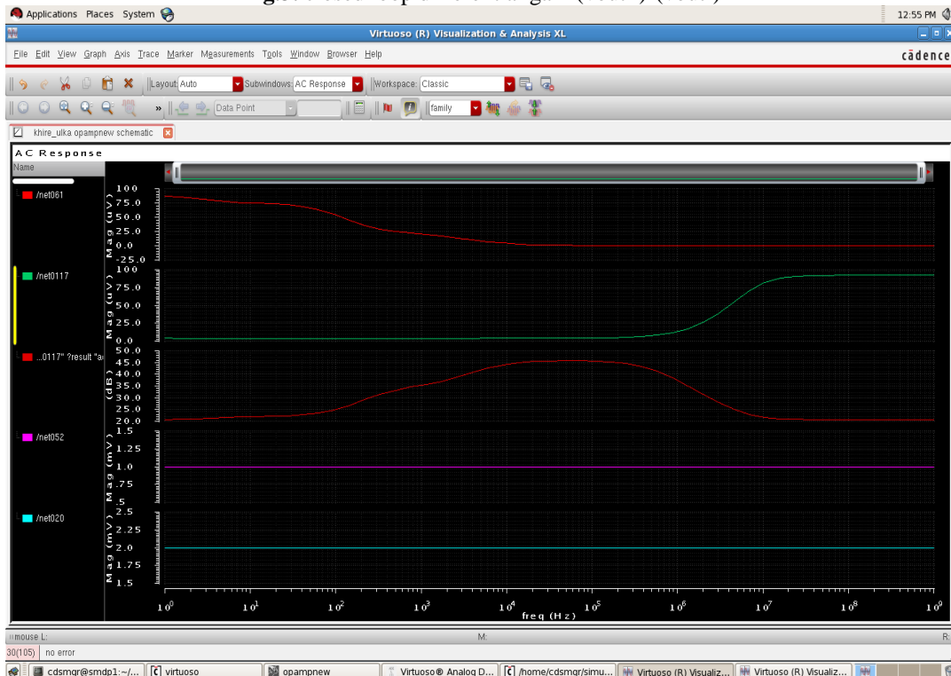
Fig.3. closed loop differential gain (vout+)-(vout-)
