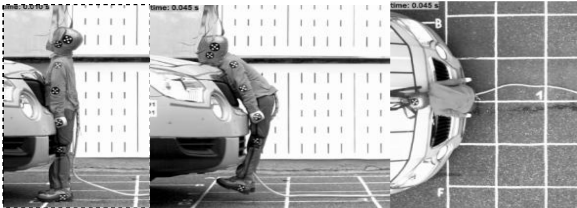
Fig. 15: Child pedestrian vs. passenger car crash configuration, from the left: the first contact, the first contact of the head with the bonnet
