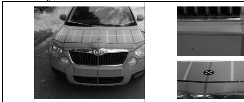
Fig. 13: Vehicle damage after collision - test No. 202
