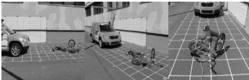
Fig. 7: Final position of objects after collision - test No. 102 – photodocumentation
