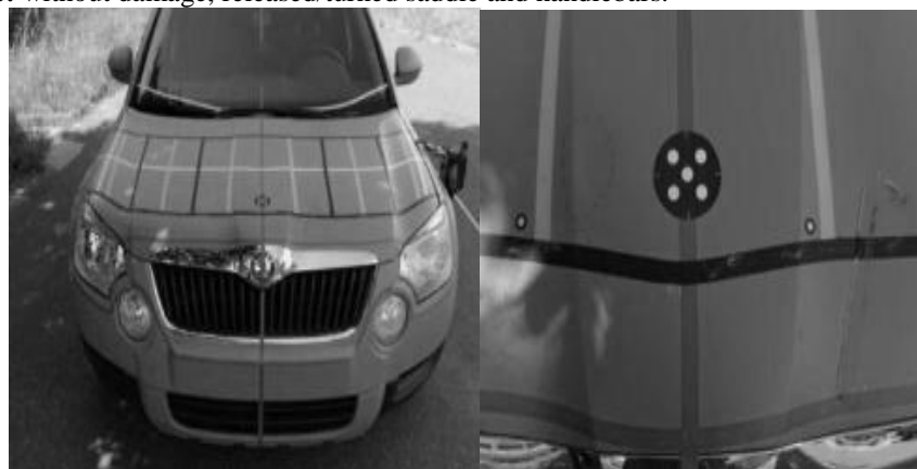
Fig. 8: Vehicle damage after collision - test No. 102
