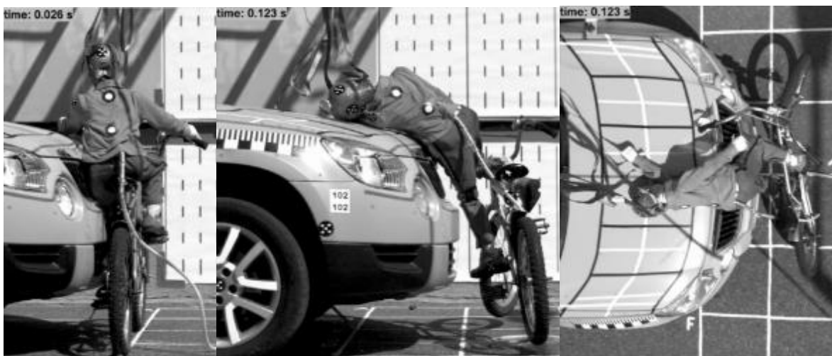
Fig. 16: Child cyclist vs. passenger car crash configuration, from the left: the first contact, the first contact of the head with the bonnet
