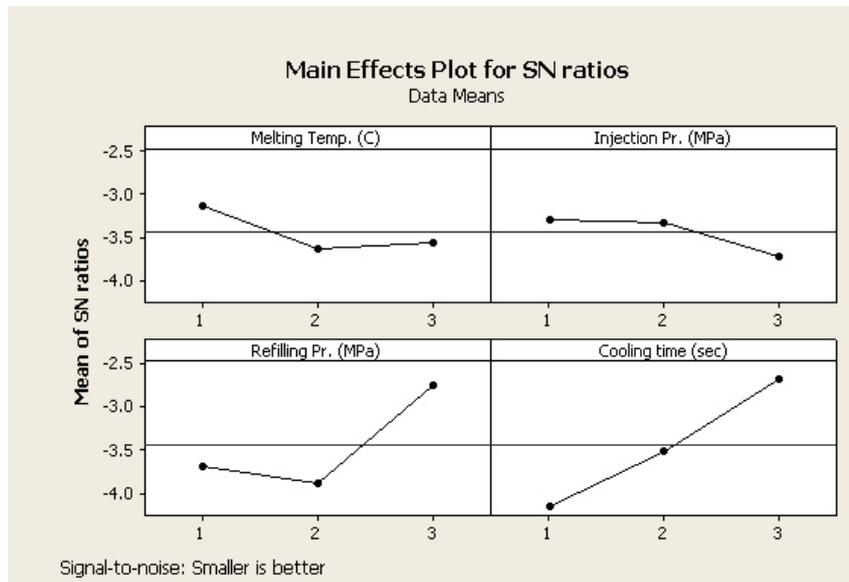
**Fig.1** Plot of Main Effects for S/N ratio
