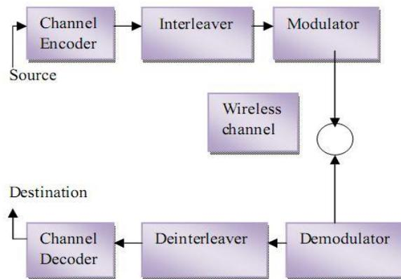
**Fig.3:** A general communication system diagram.
