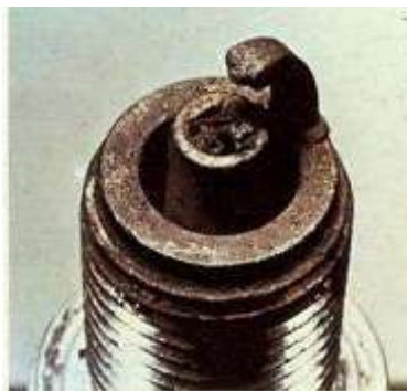
Fig.4: Overheating of Spark Plug
