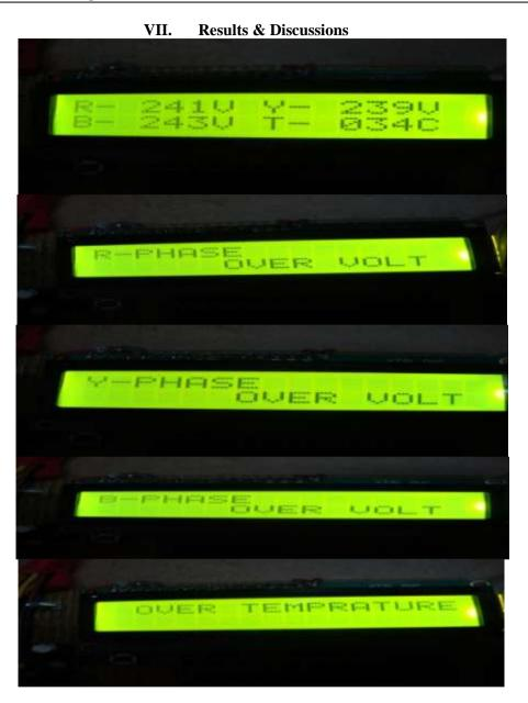
We have manually made faults on every phase and made the system to trip the circuit. When R phase's voltage become more than rated value, our system identified the fault and tripped the circuit. And at that time LCD was showing R PHASE OVER VOLTAGE.
