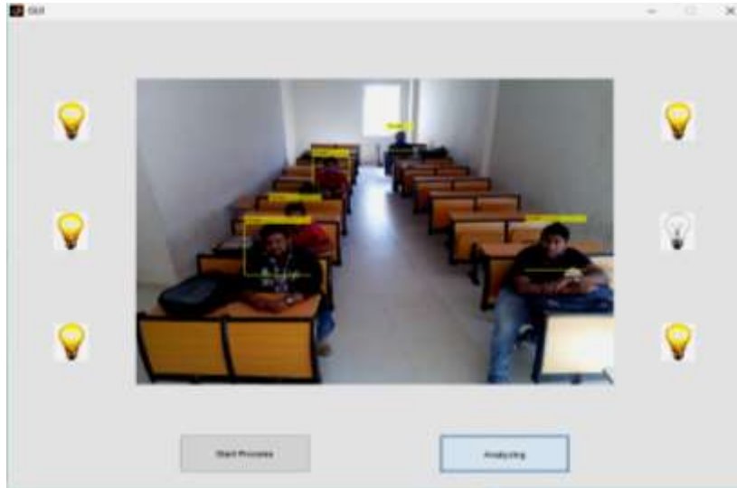
Fig. 10: Equipments Controlled According to Detected Faces
