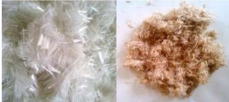
Figure: 1 Photographic Image of Prepared Glass and Jute fiber for Hybrid Composites
