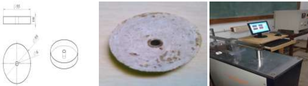
Figure: 2 Photographic Image of Composite Specimen and Pin-On-Disc Tribo Test Machine
