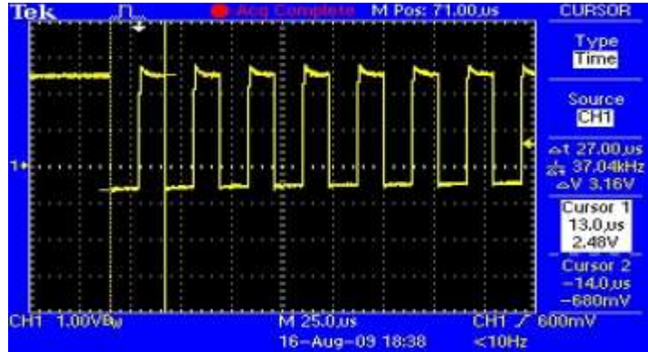
Fig. 6: Infrared signal on a Digital Cathode Ray Oscilloscope(Magnified)
