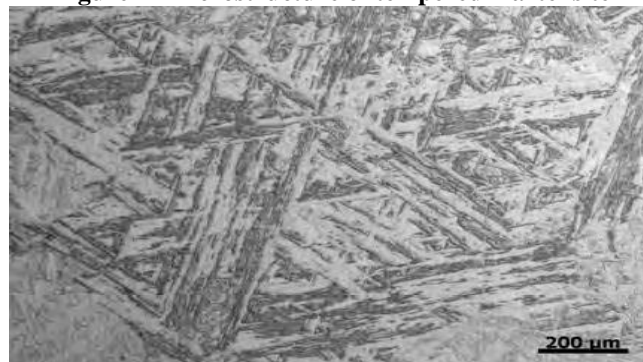
Figure 1- Microstructure of tempered martensite
