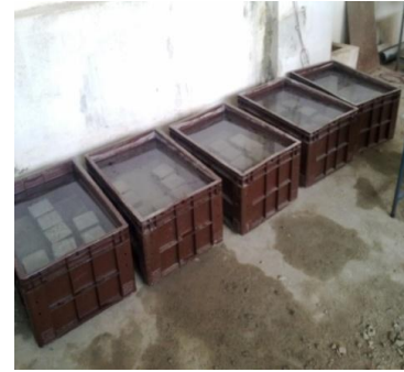
Fig 4. Cured in Sulphuric acid ( H_2SO_4 ) Solution
