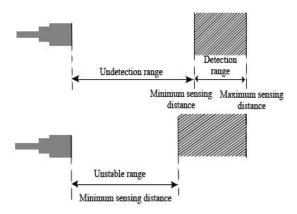
The Undetection zone is the area close to the sensor where detection is not possible due to the sensor head configuration and reverberations. Detection may occur in the uncertainty zone due to multi-reflection between the sensor and the object.
