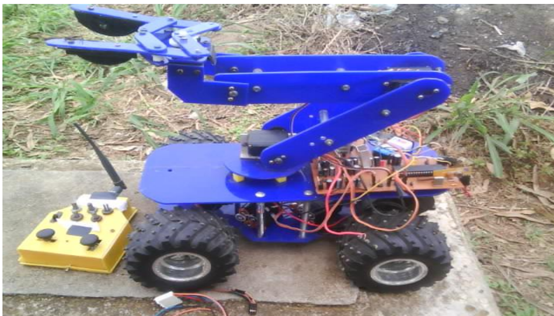
Fig. 13: Side View of the prototype “ Remote Controlled Robotic Vehicle
