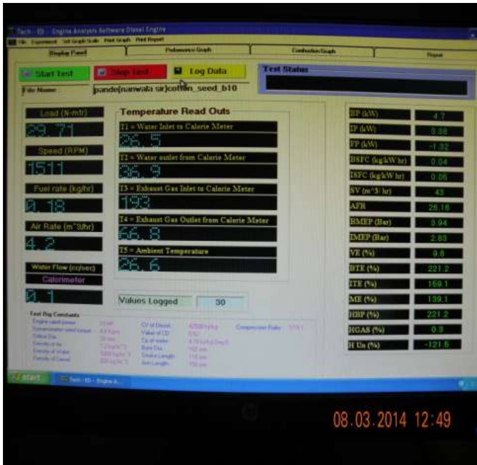
Fig 8:-Performance Test Reading by Computerized DA System
