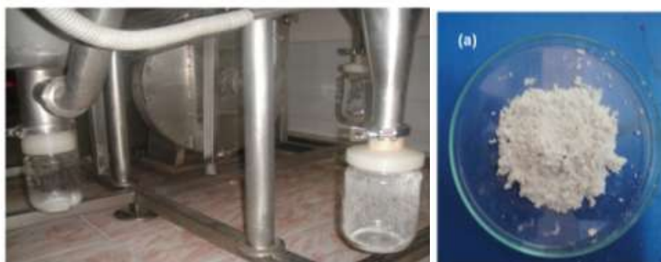
Figure 1. Encapsulated oil powder being collected in glass bottles mounted at the bottom of the drying chamber and cyclone separator. (a) Encapsulated nutmeg essential oil powder
