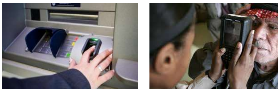
Fig.2: Finger vein and Eye vein imaging systems
