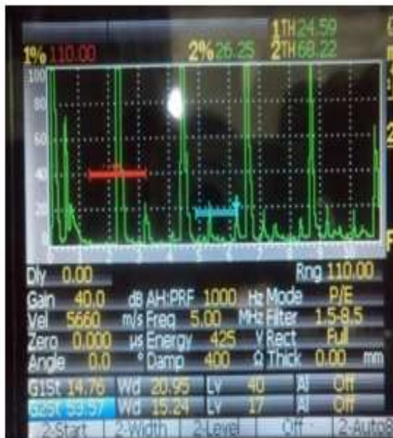
Fig-3 Ultrasonic CRT screen for defect Location 1
