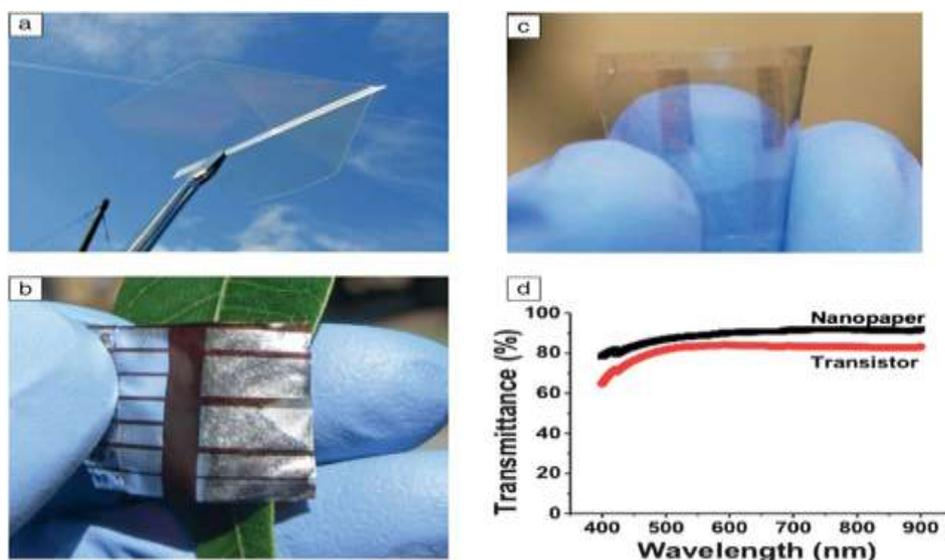
**Figure 5.** (a) Transparent nanocellulose paper made of cellulose nanofibers © 2009 Wiley-VCH Verlag GmbH & Co. KGaA, Weinheim. (b) An organic photovoltaics device on transparent nanocellulose paper © 2013 Royal Society of Chemistry. (c) A picture of a transparent and flexible nanocellulose paper transistor. (d) Comparison of the optical transmittance of nanopaper and a nanopaper transistor © 2013 American Chemical Society.
