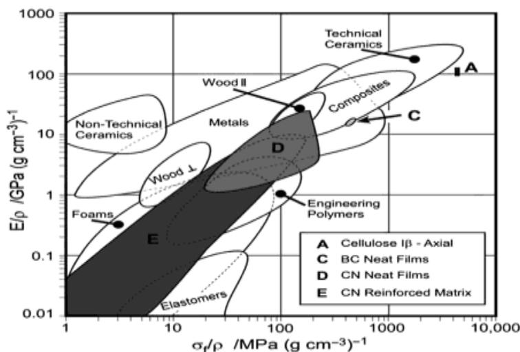
**Figure 6.** Ashby plot of specific modulus ( $E/\rho$ ) versus specific strength ( $\sigma_f/\rho$ ) © 2011 Royal Society of Chemistry.
