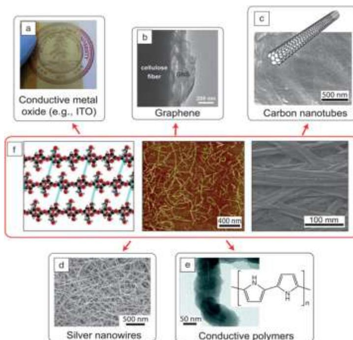
**Figure 2. Diagram showing conductive materials, such as (a) tin doped indium oxide (ITO) © 2013 Royal Society of Chemistry. (b) Graphene © 2011 Wiley-VCH Verlag GmbH & Co. KGaA, Weinheim. (c) Carbon nanotubes and (d) silver nanowires © 2009 National Academy of Sciences. (e) Conductive polymers © 2009 American Chemical Society, can be integrated into cellulose at different scales (f), ranging from the molecular level to nanofibrils, and the microfibril level.**
