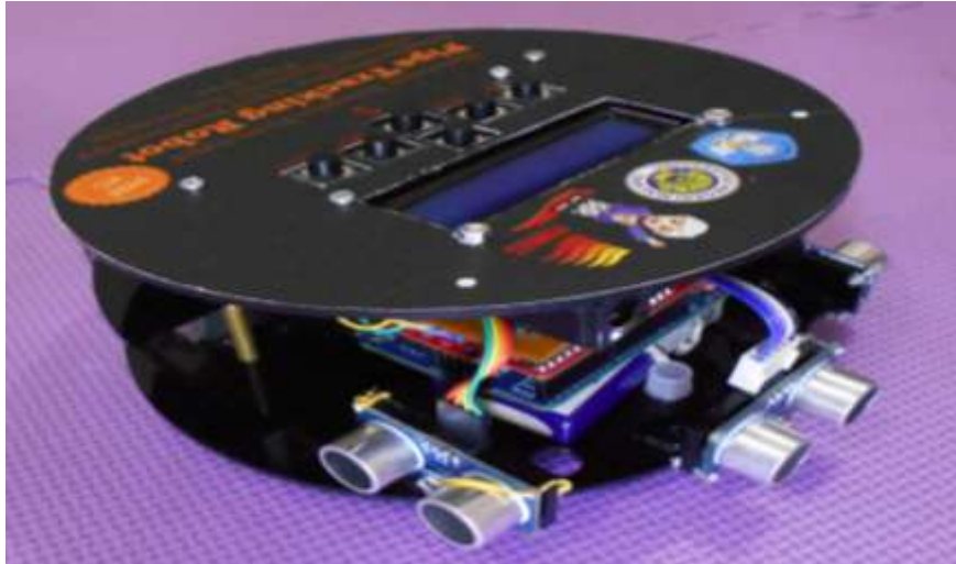
Fig. 2: The prototype of the pipe tracking robot
