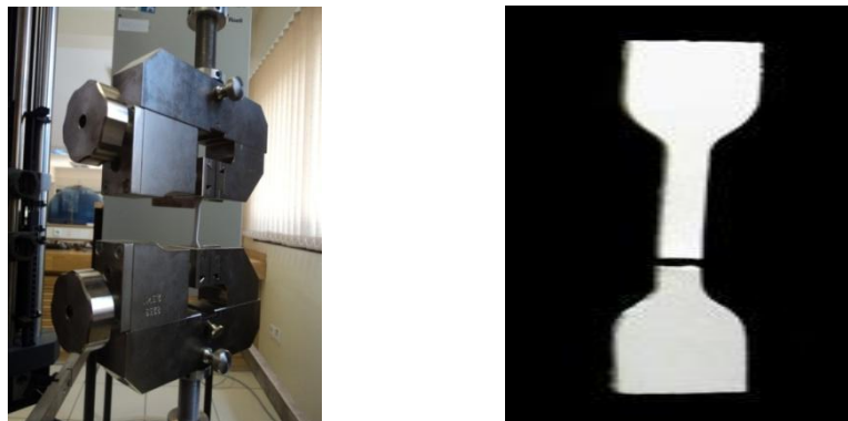
Figure 1: Test piece dumbbell during a tensile test (left), Rupture of a dumbbell specimen types ASTM D638-03 after static tensile test (right)
