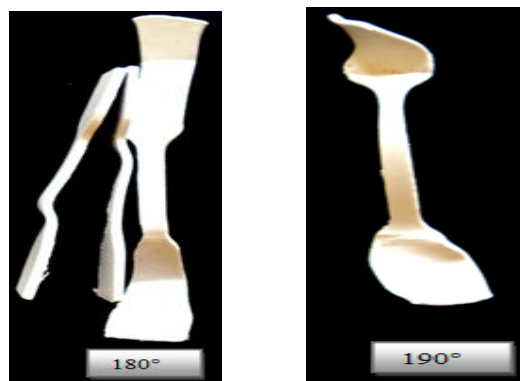
Figure 4 specimens after tensile test at temperatures above 170 \text{ } ^\circ\text{C}
