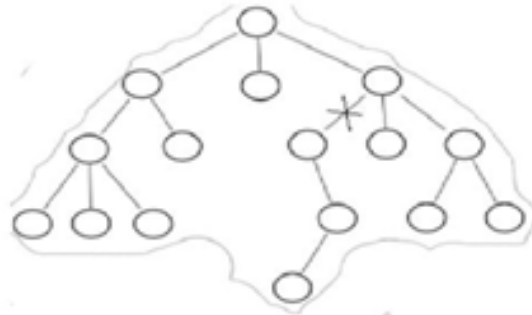
Fig 3: Link Failure and Node
