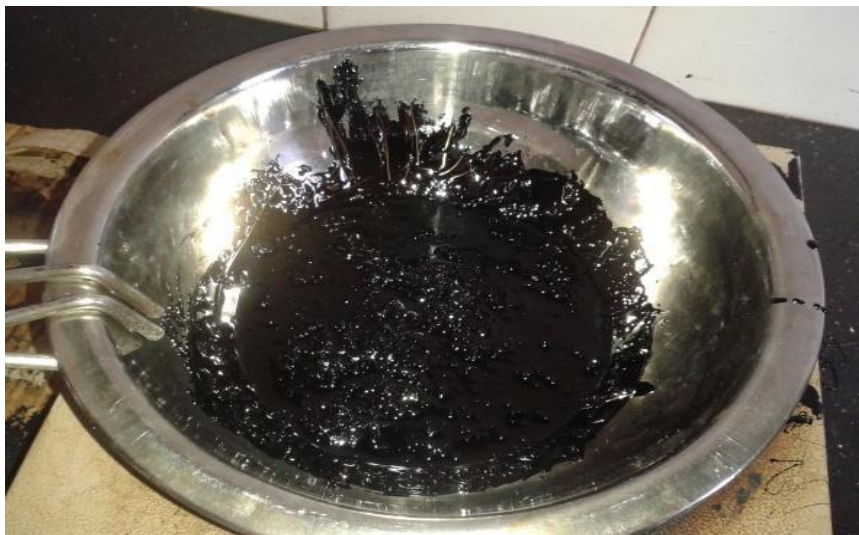
Fig.2. PP Fibres mixed with bitumen
