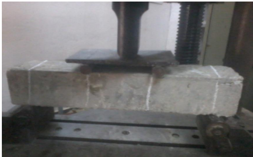
Plate: Specimen under Flexural Strength Test
