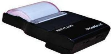
Thermal printing (or direct thermal printing) is a digital printing process which produces a printed image by selectively heating the coated thermal paper, when the paper passes over the thermal print head. Thermal printing is notable for being the only form of printing which involves no ink or toner. A thermal printer comprises these key components:
