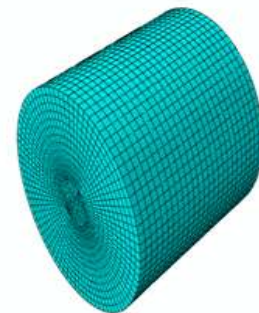
Fig 6. Meshed crack tip region
