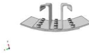
Fig 4. 3D FE model of curved stiffened panel
