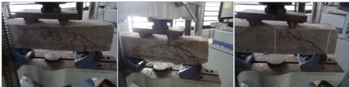
Fig. No. 5: crack pattern for B1, B2, B3 beams without shear reinforcement
