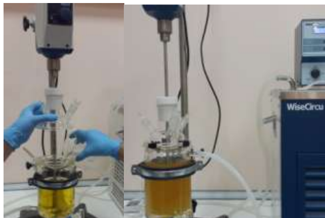
Fig.7: Adding the mixture in the reactor (B1)
