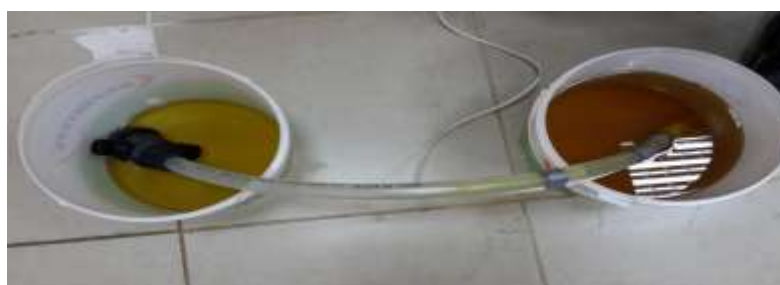
Fig.3: The filtration process of waste oil
