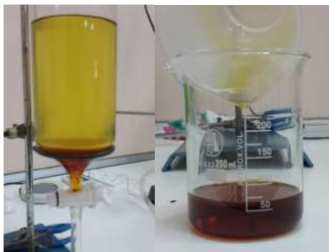
Fig.8: The glycerin removal process
