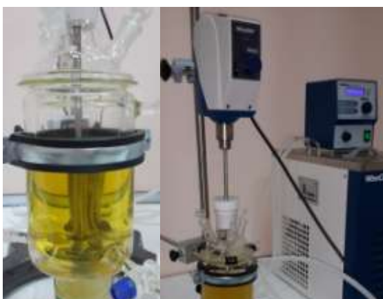
Fig.11: Preparation of catalyst and methanol mixture
