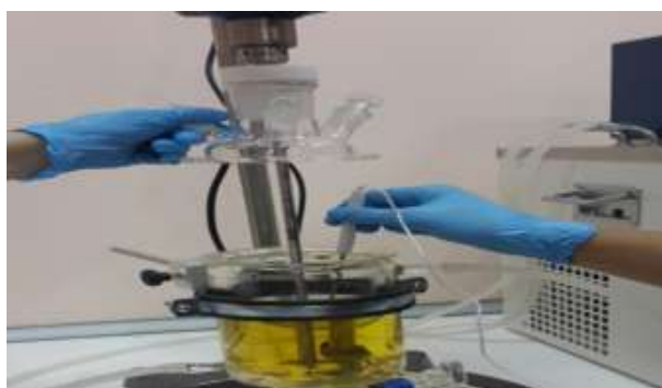
Fig.5: Preheating phase of waste oil
