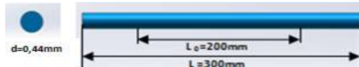
Fig. 3: Dimensions of the studied wire
