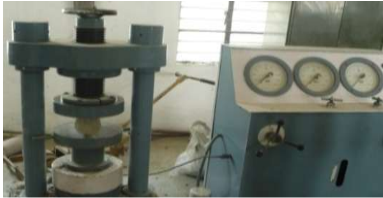
Figure3 Testing of Cylinder for Split Tensile Strength Test
