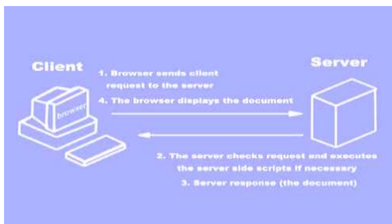
Figure 1. Client-server architecture for the server-side scripting technology
