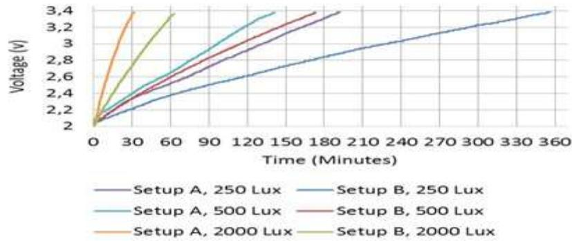
**Fig. 3.** Charging rate comparison between Setup A and B
