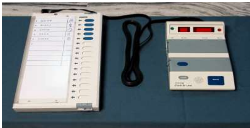
Fig. 1 Control Unit (right) and Ballot Unit (left) in the Indian EVM [3].
