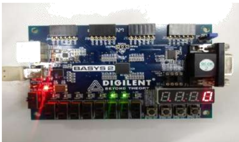
Figure 12: 'renable=1' when 'empty=1' condition is reached, results in 'underflow=1'
