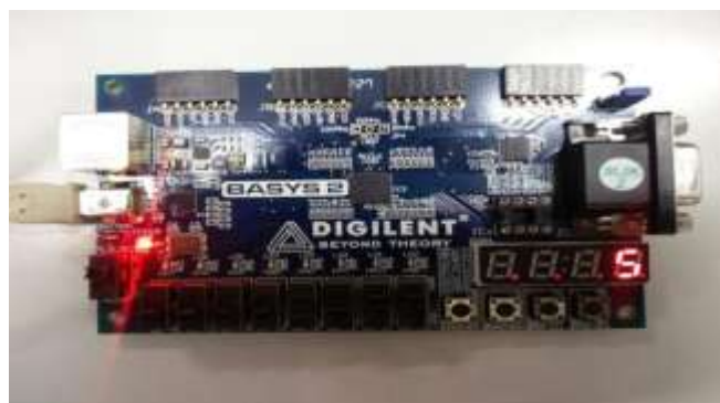
Figure 14: 'seven segment display' showing 'data_out' from the FIFO.
