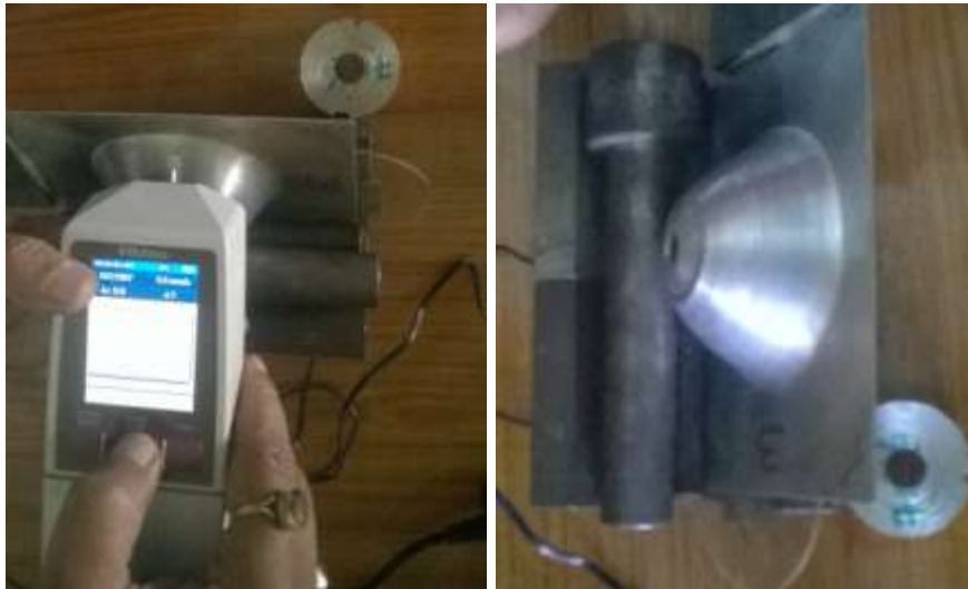
Fig. 3: Surface roughness measurement of specimen
