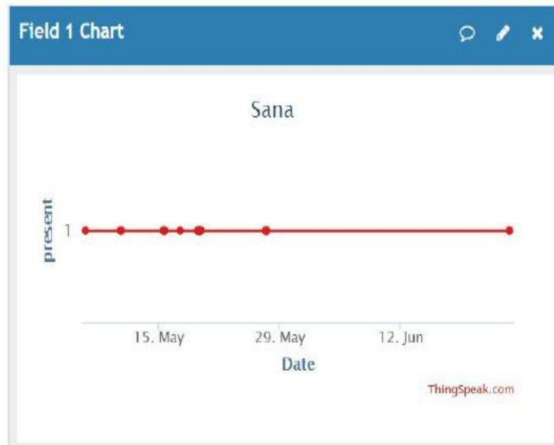
Fig 12: Details of channels created and display of student attendance on ThingSpeak
