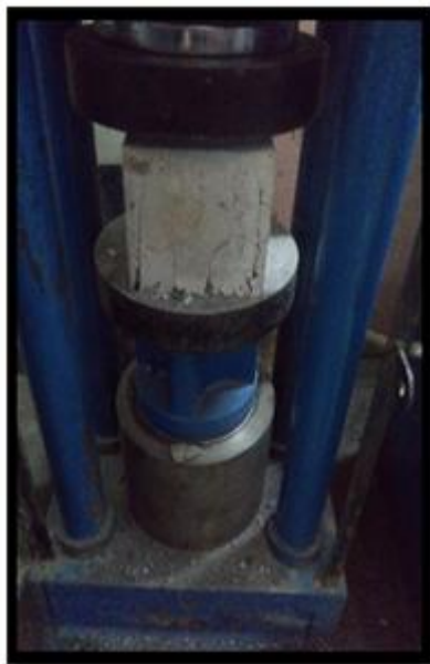
Figure 3.1 : Compressive strength on cube specimen
