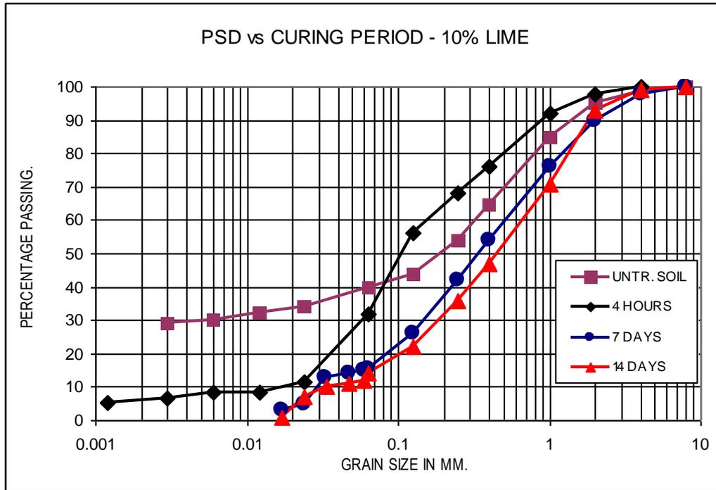
Fig. 5: Effect of curing time on PSD of lime-treated clayey SAND for 10% lime content
