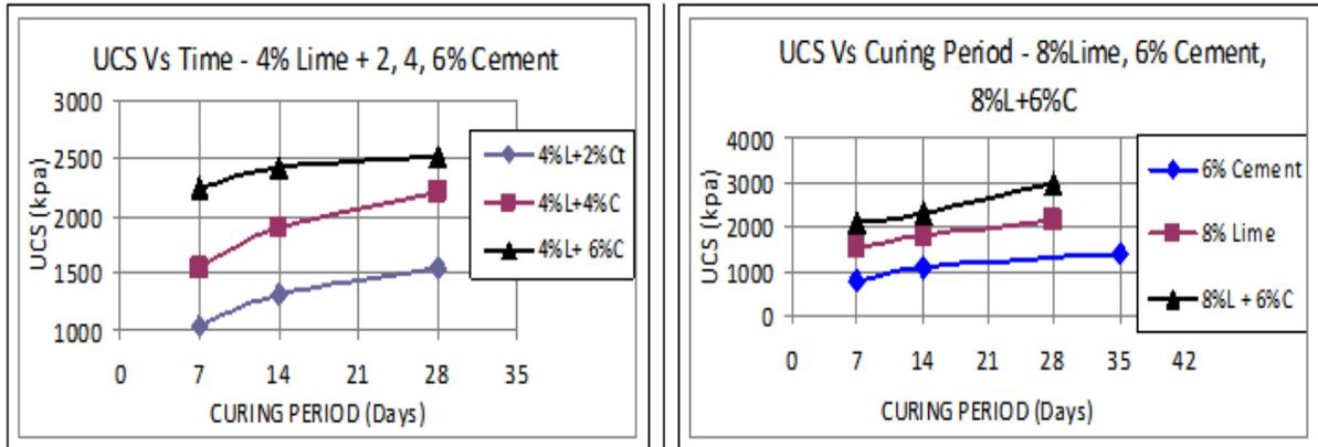
**Fig. 7:** UCS development with time and lime-and-cement content in two-stage stabilization of clayey SAND
