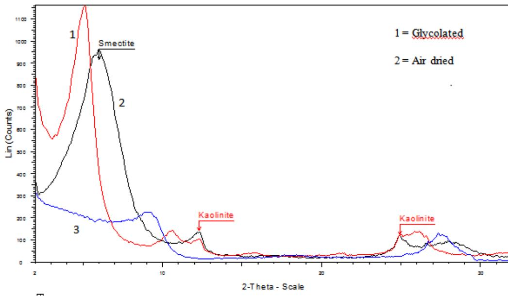
Fig. 3: Mineralogical analysis of the clay fraction (by XRD)
