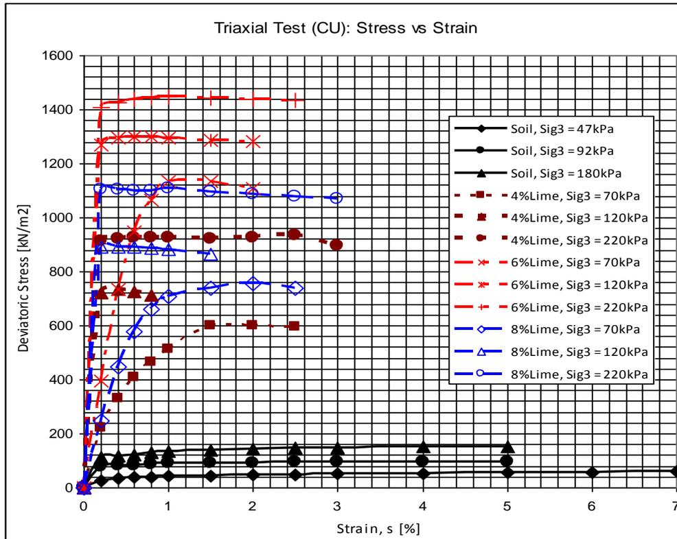
Fig. 7: Results of CU triaxial compression on natural and lime-treated soil samples
