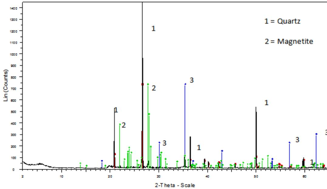
Fig. 2: Mineralogical analysis of Kibaha expansive soil (by XRD)
