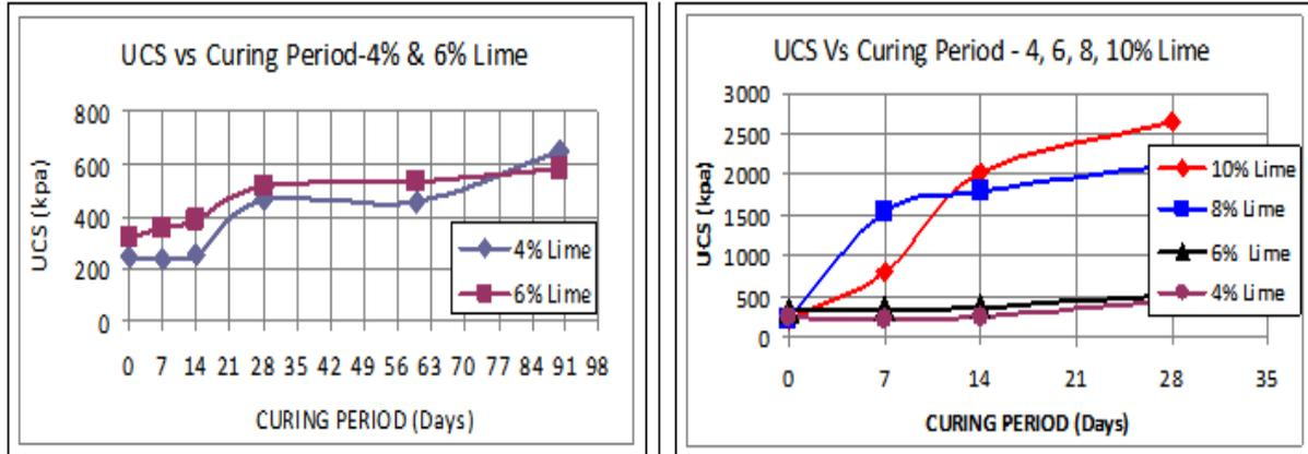
**Fig. 6:** Effect of lime content and curing period on unconfined strength of lime-treated clayey SAND
