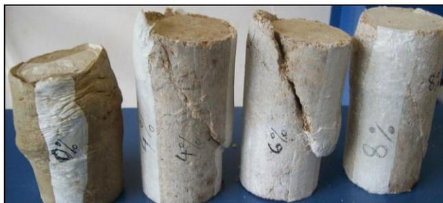
**Fig. 6:** Triaxial compression (CU) samples after test
