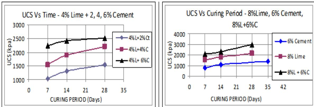
**Fig. 7:** UCS development with time and lime-and-cement content in two-stage stabilization of clayey SAND
