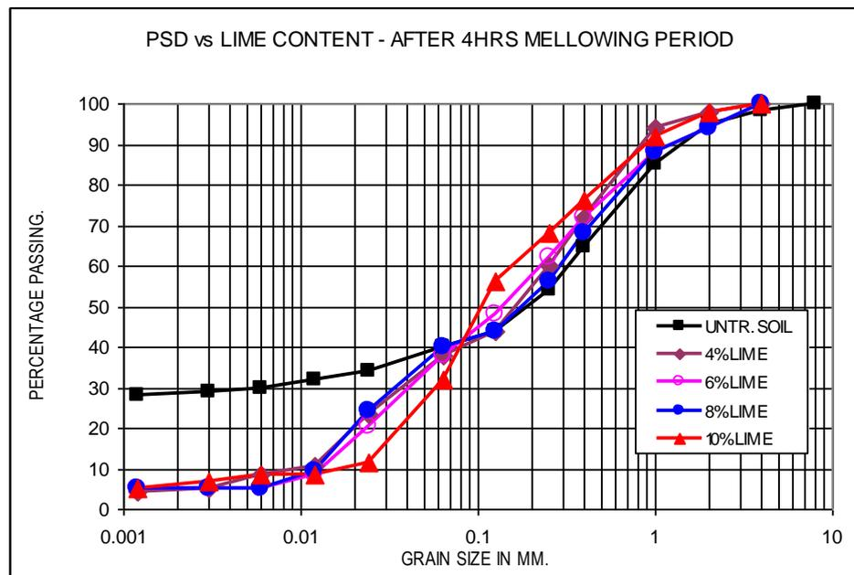
Fig. 4: Effect of lime content on PSD of lime-modified clayey SAND
