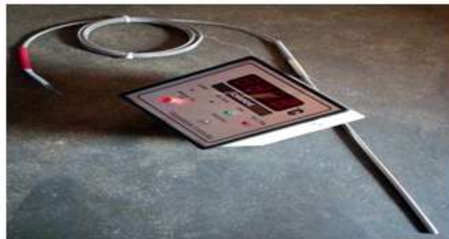
Fig.9. K Type Thermocouple and temperature indicator
