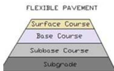
Figure 3.1. Pavement Construction Layer
