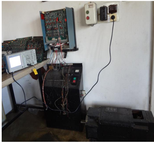
Fig. 4: Experimental study of a spindle electric drive.
