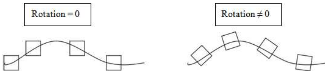
Figure 8. Potential flow vs rotational flow.
